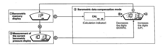
Use this mode for making compensation to the barometric data of the watch by adjusting the standard barometer..
