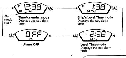
The alarm mode change in the order shown above each time the ⓐ button is pressed and relased while in the normal Alarm mode.
