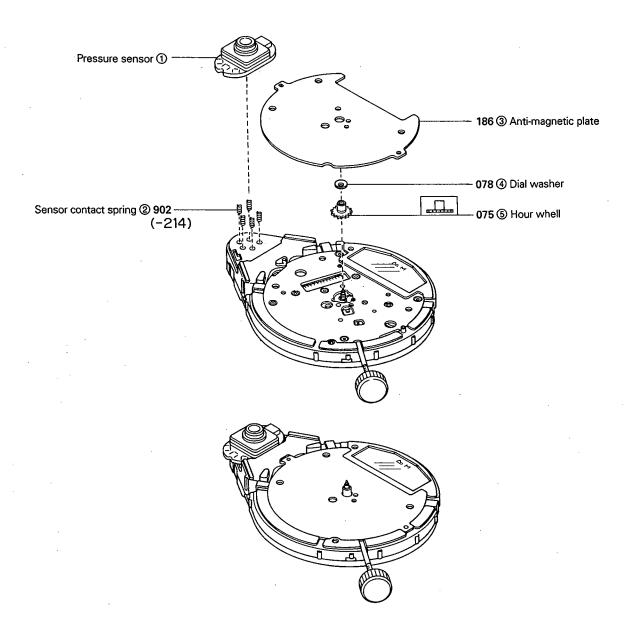
**Note:** Anti-magnetic plate has directional properties. If it is inverted, dial cannot be mounted.
