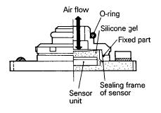
The sensor is protected by gel material as shown in the figure at left. Never stick it with a bar.
